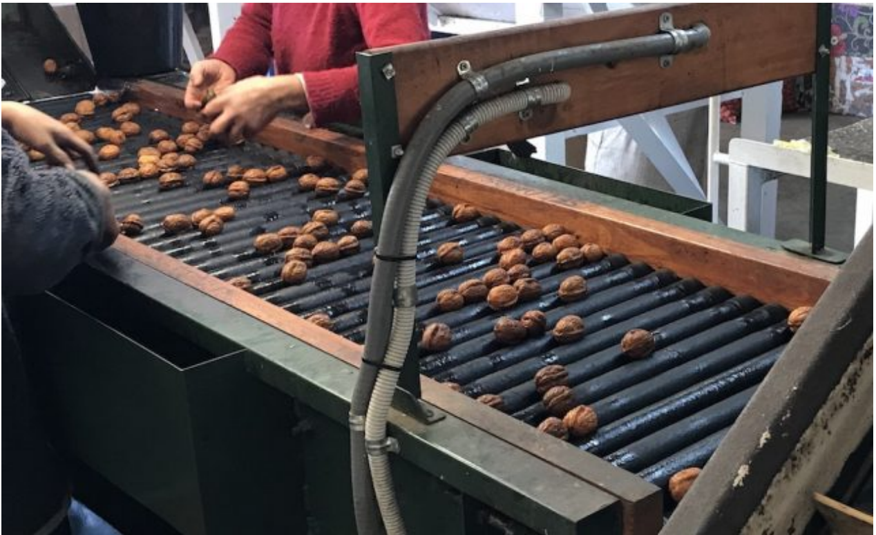
Duds are removed by hand on the sorting conveyor
